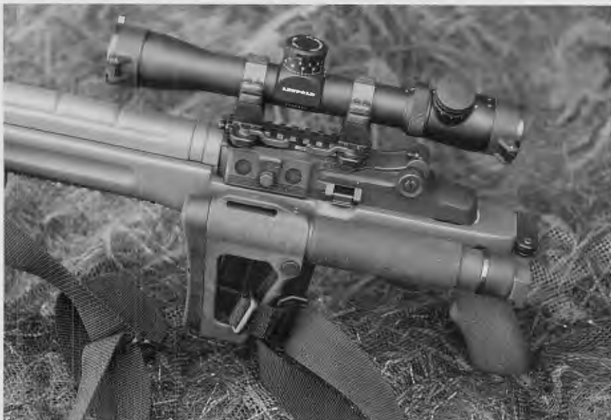
On the A.R.M.S. #18 is mounted the Leupold MR/T 3-9x36mm Tactical Scope, the civilian version of the Army's Leupold TS-30A2 Sniper Scope.
