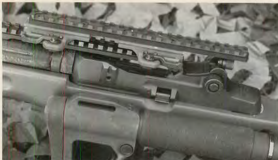
To accommodate special eye-relief problems, a MOA Solution rail locks onto the Ross Rail allowing it to extend to the rear for night vision scopes.
