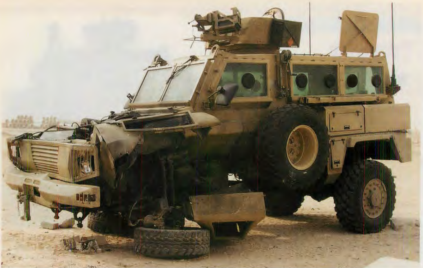
An RG-31 Cougar rests on its front axle after an IED detonated under the vehicle. None of the Marines were seriously injured and the vehicle was repaired. Photo courtesy of 8th Engineer Battalion.
